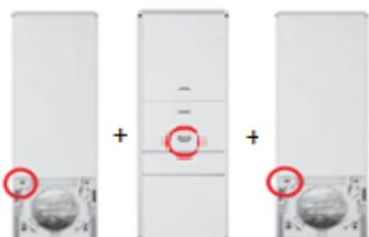
Press 1x **P2 button**, 1x **down button** and 1x **P2 button**. The drive confirms as always with a beep and an up/down movement. At the end, the drive confirms with several beeps. Both end positions are now deleted. You can set new end positions now.
