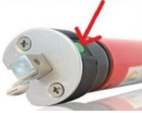
Press and hold the **learn button** on the motor head with an object until the drive reacts only 3 times with a up/down movement and 3 beeps. Release the **learn button** again. The motor is now set to the factory settings. All previous connections and settings are deleted.
