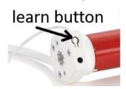
Press and hold the **learn button** on the motor head with an object until the drive reacts only 4 times with a short up/down movement and 4 beeps. Release the **learn button** again. The motor is now set to the factory settings. All previous connections and settings are deleted.
