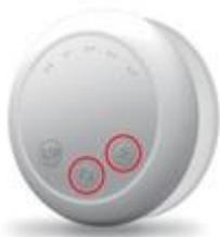
1. Press and hold the **P2 button** and the **sun button** simultaneously.
